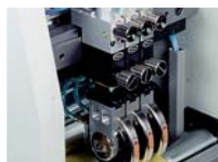
Pneumatically operated knife holders and driven bottom shaft
